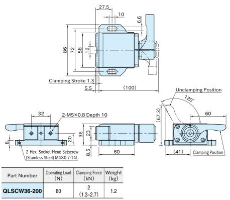
Note : The above operating load and clamping force are obtained when clamping the workpiece at the midpoint of the clamping stroke. The clamping force varies within the above range depending on the amount of compression of the spring.
