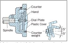
Indicators must be installed in the angular range shown above.
