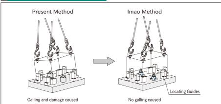
The locating pin gets projected only after the workpiece is set on supports. This allows loading and unloading the workpiece smoothly, with no galling.
